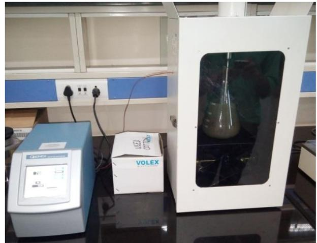
Figure: 6 Probe type ultrasonicator
